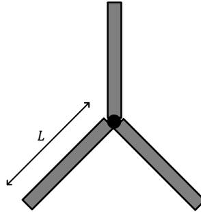
**Solution 2a:** Just as we can compute the rotational inertia of a system of point objects by summing the inertia of each object so can we find the rotational inertia of a system of continuous bodies by summing the inertia of each body. It's important to note that in both cases the axis of rotation must be the same for all objects /bodies being summed. With this knowledge, the rotational inertia of the rotor is:
