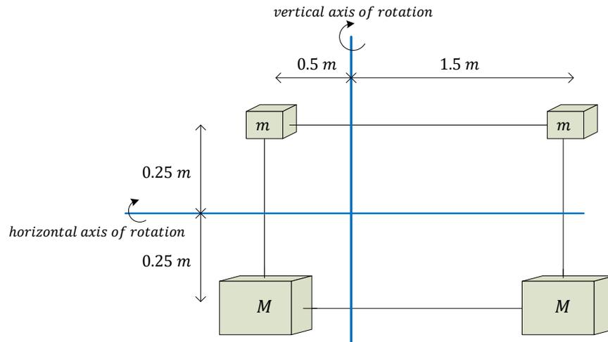
**Solution 1:** The summation formula can be used for each axis of rotation as shown.
