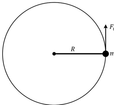
When a tangential force,  $F_t$ , is applied to the mass, it will tend to travel along the circular path because of the centripetal force being supplied by the tension in the rod. As it travels around the circle the mass is undergoing tangential acceleration, from the applied force, and radial acceleration, from the tension in the rod. Focusing on the tangential acceleration we can use Newton's 2<sup>nd</sup> law to write the following relationship.
