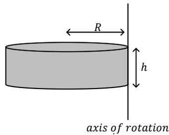
Since the new axis of rotation is oriented parallel to the center of mass axis used previously, we can use the parallel axis theorem to find the new rotational inertia. The rotational inertia with respect to the center of mass axis of rotation was found above as
