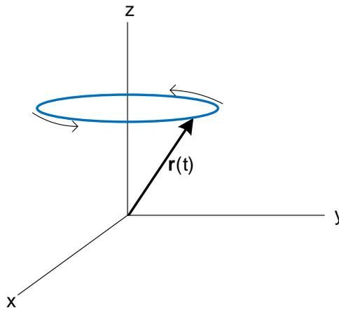
However, since  $-\infty < t < \infty$ , the path is traced in a counter clockwise direction and the vector traverses that path an infinite number of times.
